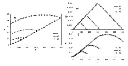
Figure 1. (a) Adsorption isotherm and three desorption scanning isotherms calculated using the DCH model. Time dependences of the (b) bulk pressure and (c) adsorbed phase concentration during adsorption-desorption processes.
