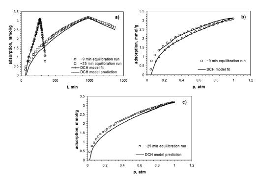
Figure 3. Carbon dioxide adsorption/desorption on microporous CFCMS activated carbon fiber at 273 K. (a) Uptake as a function of time. (b) and (c) Adsorption/desorption isotherms. Circles and squares denote experimental data for two runs with  $\sim$ 9 and  $\sim$ 25 minutes equilibration intervals, respectively. The data from  $\sim$ 9 min run were fitted with the DCH model and the equilibrium adsorption isotherm for  $\sim$ 25 min run was predicted by the model.
